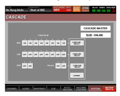
A serial PC port connection of the Master and Sub mixers is required to enable control functions of cascade mode (Mini DIN 8-pin) \*in cascade mode, PC port can not be used for any other communication mode.
