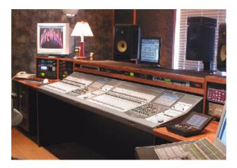
The MTBK-R109 board also enables cascade connection of two DMX-R100 units, creating a 96-channel mixer. This means that by using two DMX-R100 control surfaces, 48 faders are physically available for mixing, reducing the need to resort to repeated paging of channel faders. Cascade connection at double sample (96/88.2 kHz)rate is also supported but with half the number of channels on each mixer, so a total of 48 channels are available.
