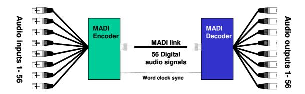
MADI can be used to transmit higher sampling rate audio signals (ie 96 kHz), there are two alternate methods specified for higher sample rate. In both methods the number of audio channels is reduced (therefore 26 mono, 96 kHz audio channels can be transmitted by MADI).
